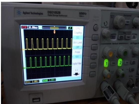
Figure 6 Stepper motor driving signal
