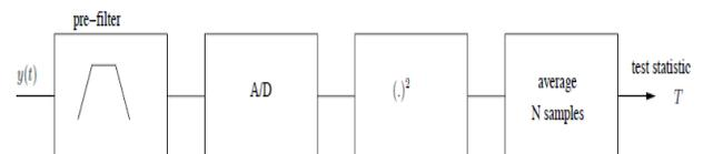
Figure 2. Block diagram of an Energy Detector.
