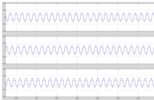
Fig.6.6 Phase Voltage from the rotor side inverter (X-axis:Time(s), Y-axis: phase voltage (V))
