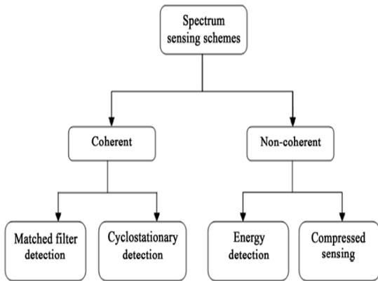
Figure 1: Types of Spectrum Sensing
