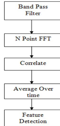
Figure 3: Block Diagram of CFD
