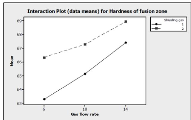
by the experimental factors. The result showed that the type of shielding gas flow rate interaction hardness in fusion zone. The pull factors that result in a hardness most argon and gas flow rate 14 l/min. Factors used in the type of shielding gas and gas flow rate of the P-Value of factors was 0.000 (<0.05). The result showed that the type of shielding gas and gas flow rate with electrification interaction significance at the maximum hardness in fusion zone at 68.97HV.
