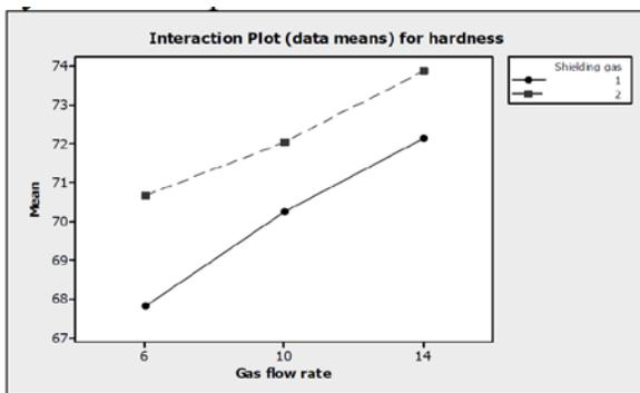
Fig. 4 Interaction plot for hardness in HAZ
