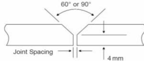
Figure 2 Joint geometry for the welding specimens
