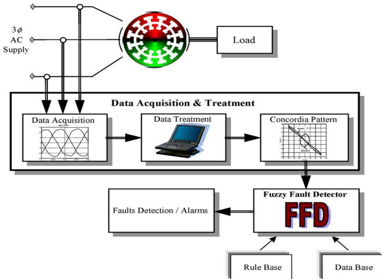
Fig. 5 The Fuzzy based Fault Detection method
