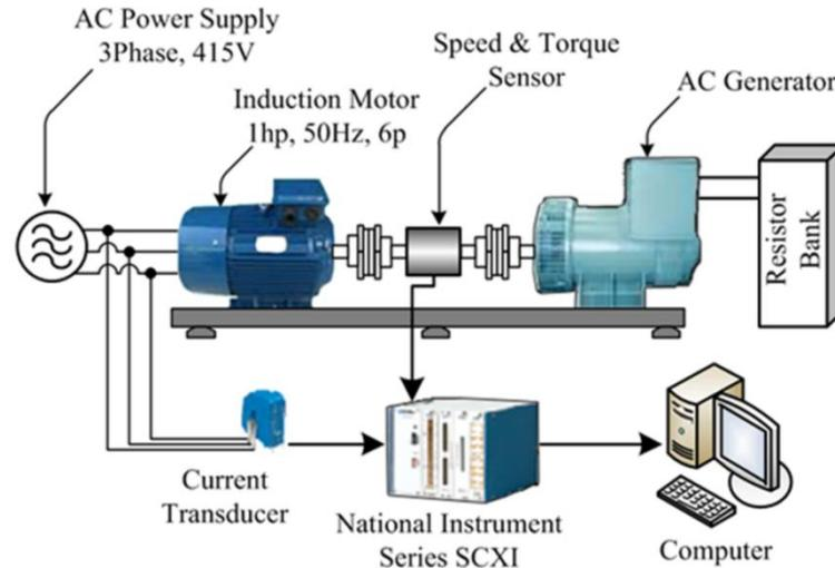
**Fig 1 –TheFault detection Setup**
