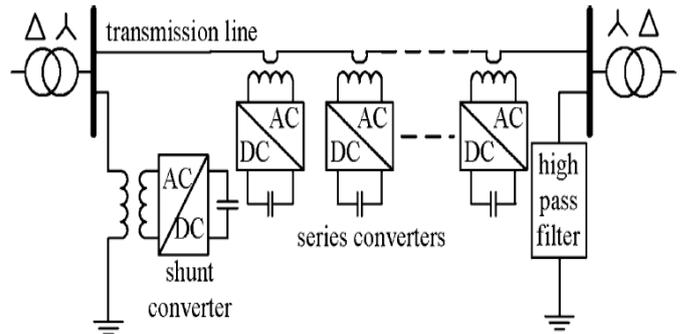
Fig 11: Distributed power flow controller (DPFC)
