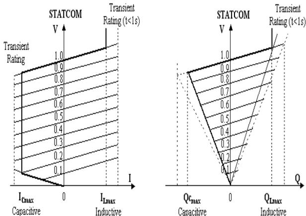
Fig 7: V-I and V-Q characteristics
