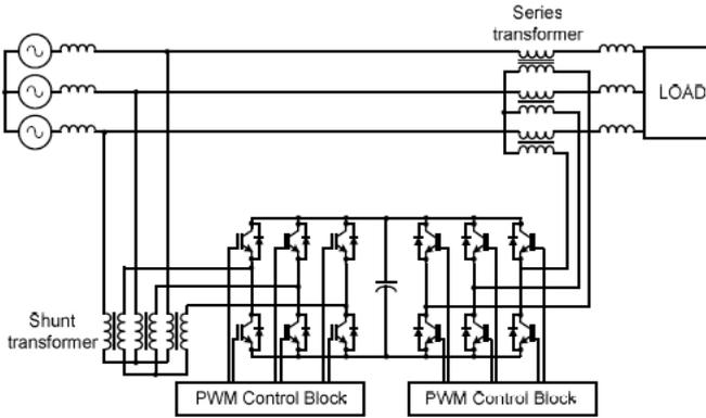
Fig 10: Unified Power Flow Controller
