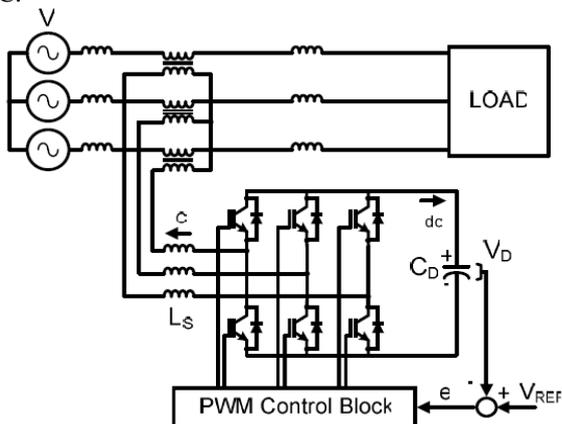
Fig 8: Static Synchronous Series Compensator
