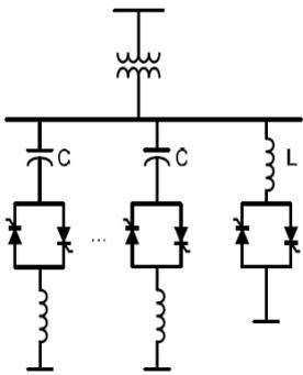
Fig 3 : Combined TSC and TCR Configuration
