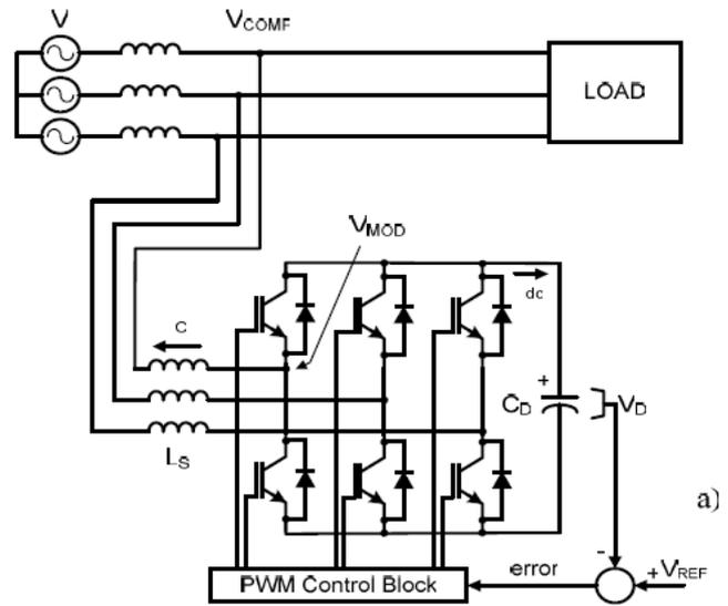
Fig 6: Static Synchronous Compensator
