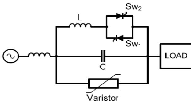
Fig 5: Thyristor Controlled Series Compensator (TCSC)
