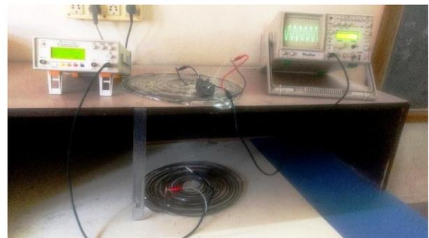
**Figure 2: Complete experimental setup for tuning of receiving coil in strongly coupled magnetic resonance based wireless power transfer system.**
