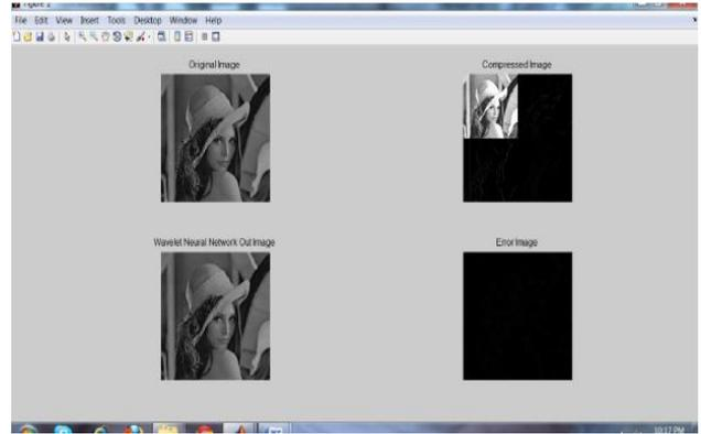
Figure 12: Image compressions by MLP with wavelet coefficients (75% compression)
