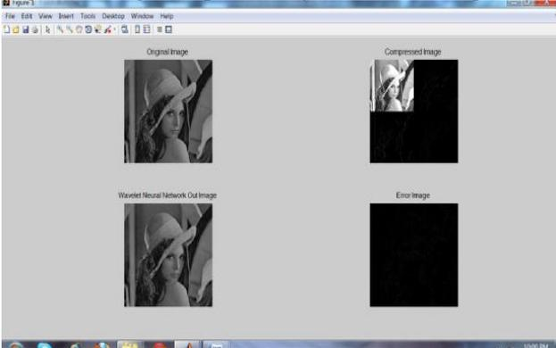
Figure 10: Image compressions by MLP with wavelet coefficients (50 % compression)
