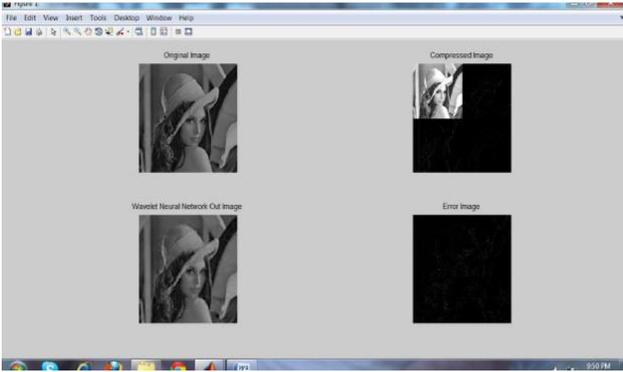
Figure 8: Image compressions by MLP with wavelet coefficients (25% compression)
