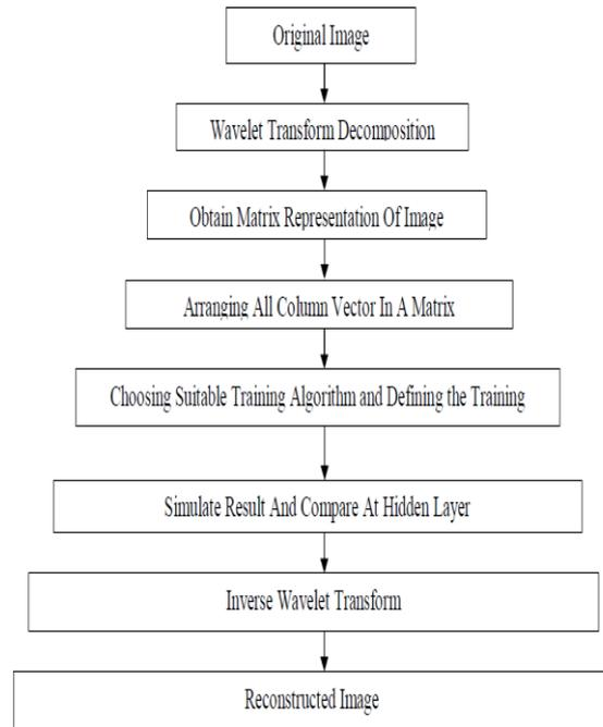
Figure 5: Flow chart for Image Compression by MLP with WT
