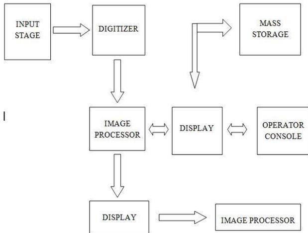
Figure 1: Elements of a Digital Image Processing System
