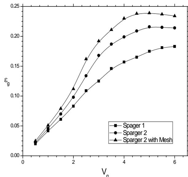
Fig. 2: Gas hold up in bubble column.
