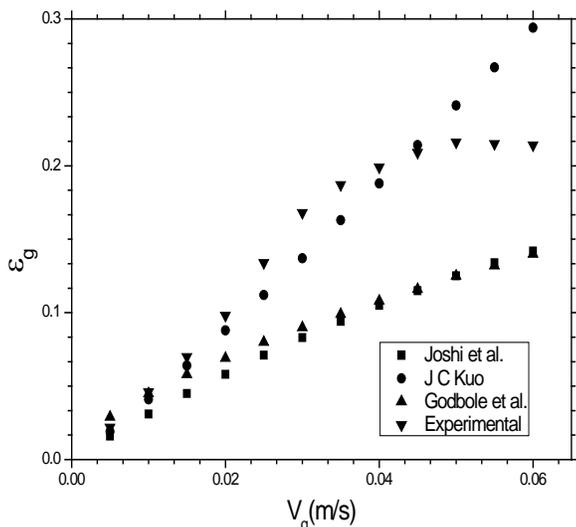
Fig. 3(b): Comparison of experimental and empirical gas hold up with Sparger-2
