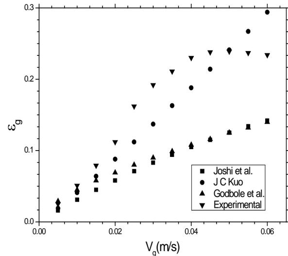
Fig. 3(c): Comparison of experimental and empirical gas hold up with Sparger-2 and mesh plates.
