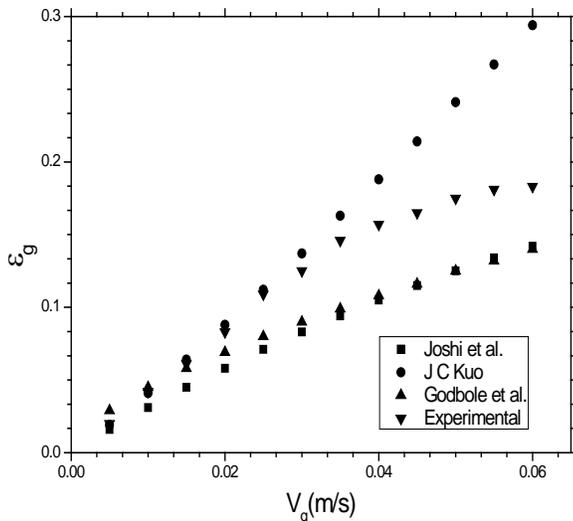
Fig. 3(a): Comparison of experimental and empirical gas hold up with Sparger-1
