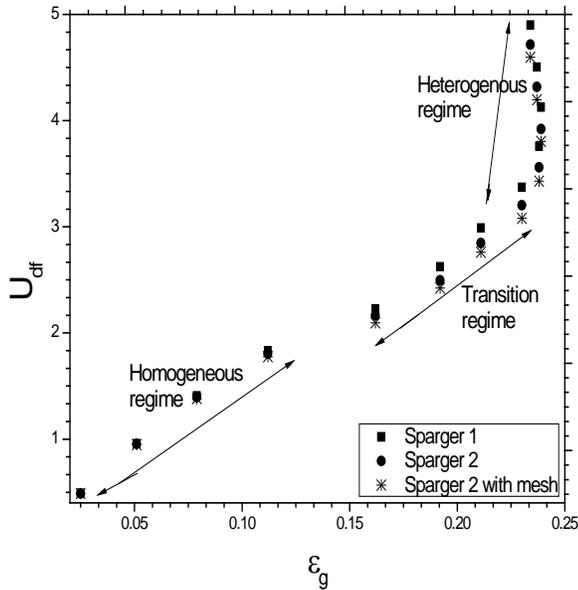
Fig. 4: Characterization of regime transitions with the drift-flux model.
