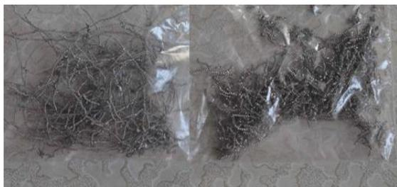
Conical Chip Tubular chip
