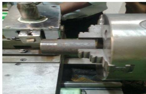
**Fig.2 Work piece Setup**
