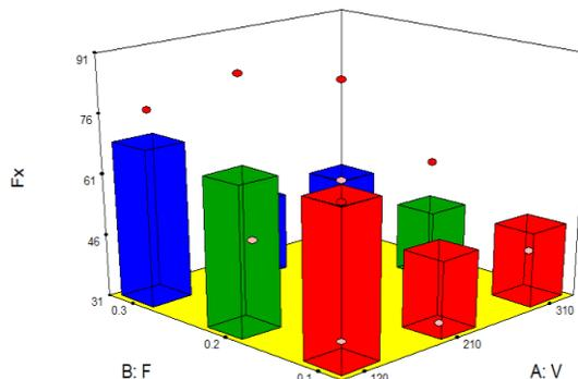
Fig. 5. 3D Solid plot of  $F_x$  effect factor V&d
