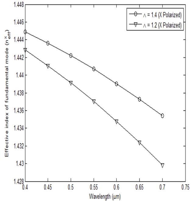
Figure 6 : Effective index as a function of wavelength for the two values of pitch (1.2 and 1.4) and X polarization.
