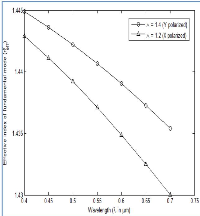
Figure 5: Effective index as a function of wavelength for the two values of pitch (1.2 and 1.4) and Y polarization
