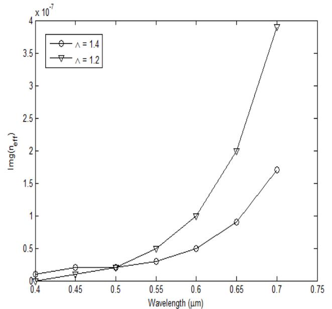
Figure 7: Imaginary part of the effective core index showing the losses in the propagation for different pitch values of the design
