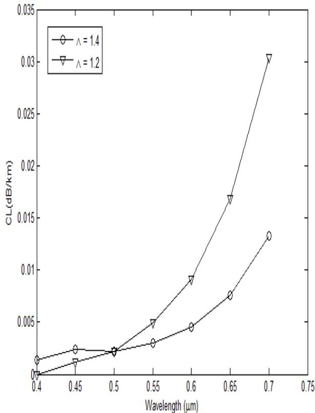
Figure 8: Confinement loss V/s wavelength
