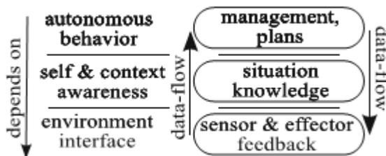
Figure 1: Essential dependencies and data-flow for autonomic computing systems
