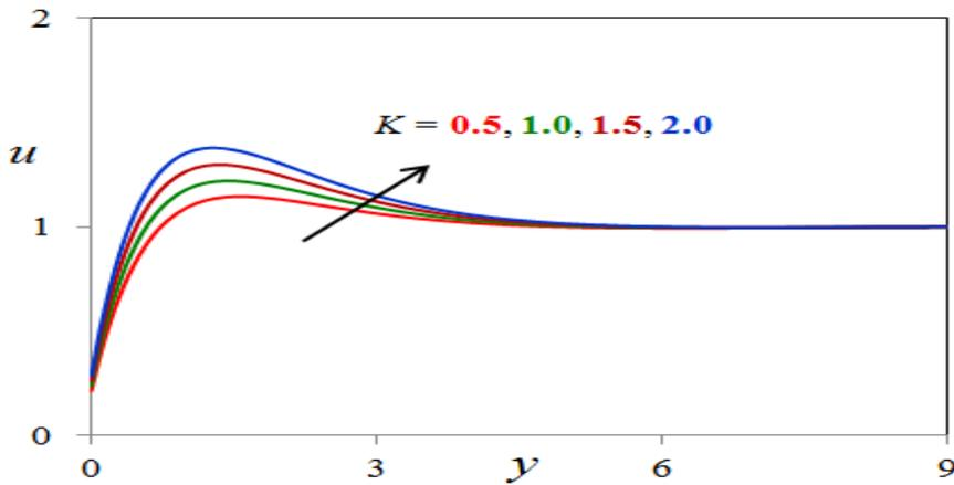
Fig. 5.  $K$  effect on velocity profiles
