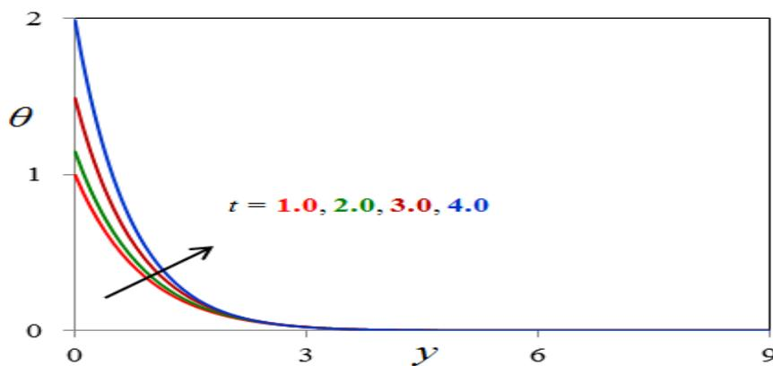
Fig. 17.  $t$  effect on temperature profiles
