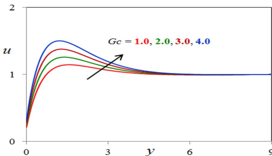
Fig. 3.  $Gc$  effect on velocity profiles
