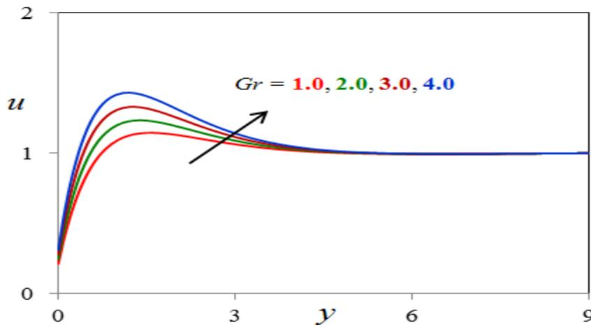
Fig. 2.  $Gr$  effect on velocity profiles
