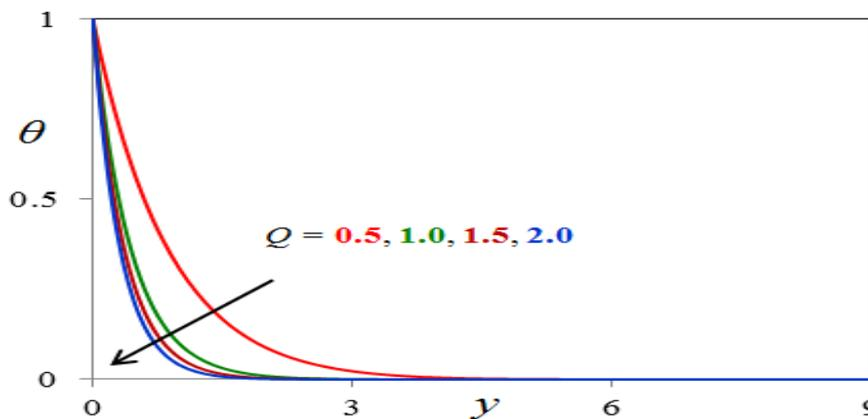
Fig. 11.  $Q$  effect on temperature profiles
