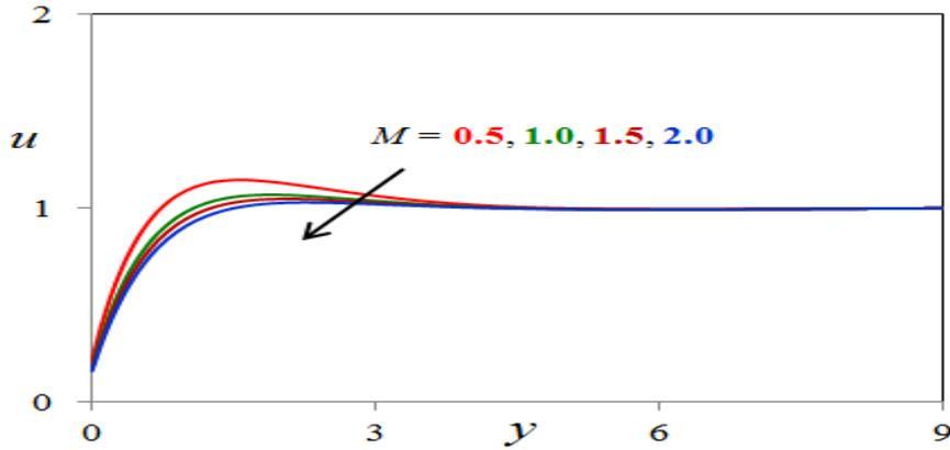
Fig. 4.  $M$  effect on velocity profiles
