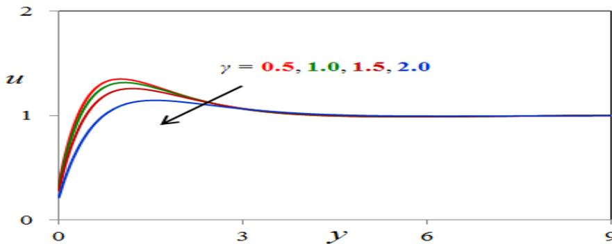
Fig. 6.  $\gamma$  effect on velocity profiles
