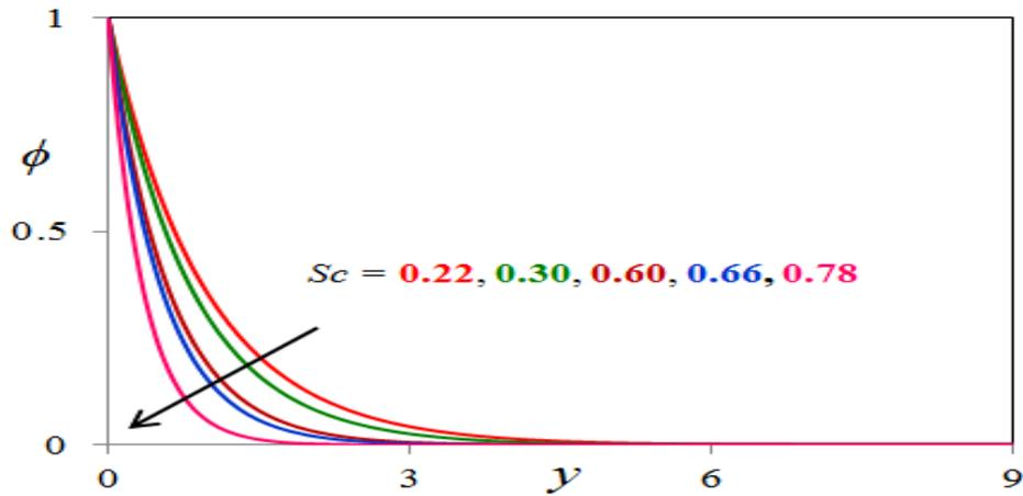
Fig. 15.  $Sc$  effect on concentration profiles
