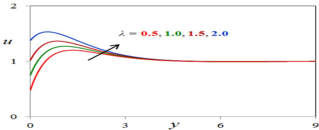
Fig. 16.  $\lambda$  effect on velocity profiles
