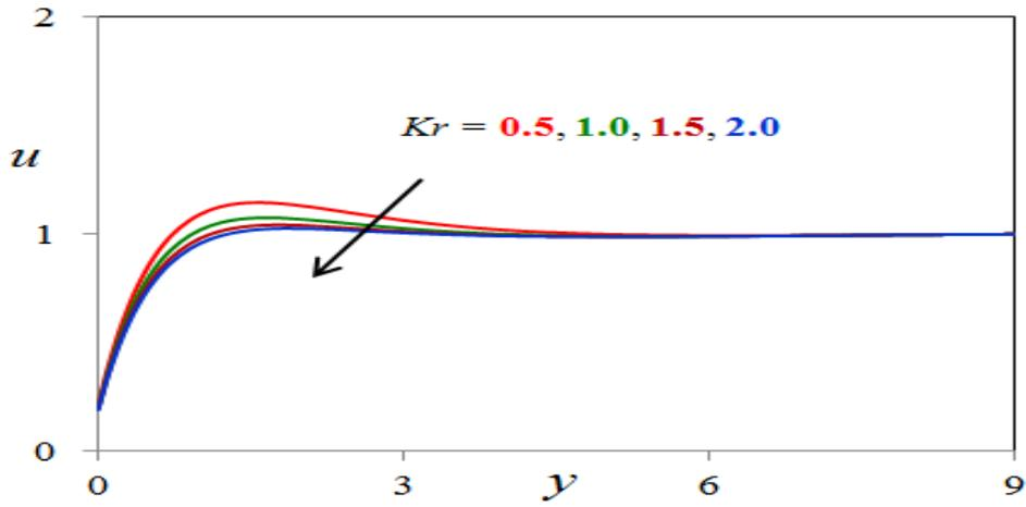
Fig. 12.  $Kr$  effect on velocity profiles
