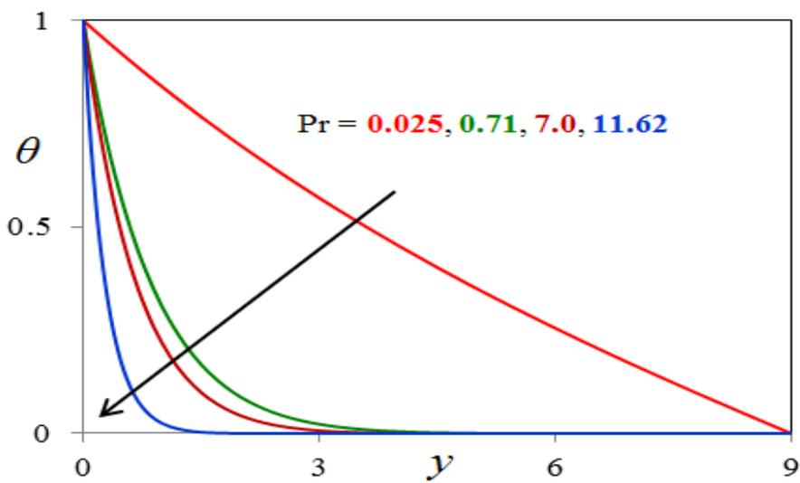
Fig.14.  $Pr$  effect on temperature profiles
