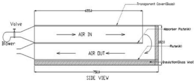
Figure 2 Double pass solar air heater
