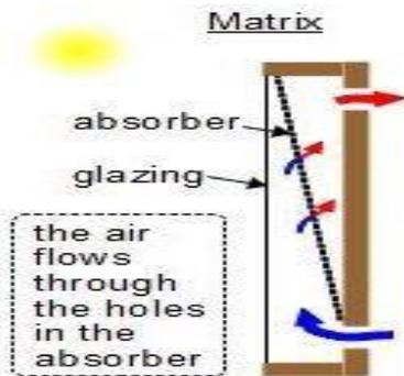
Figure 3 Matrix type solar air heaters
