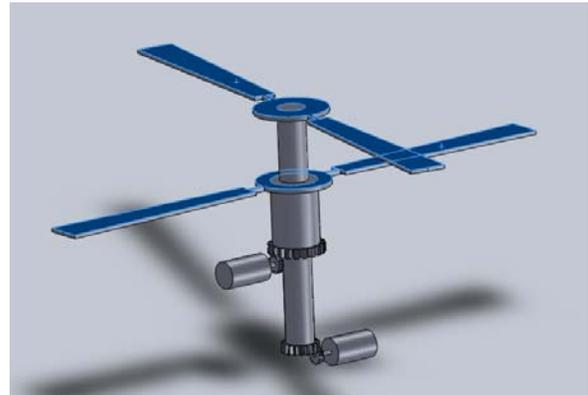
The following design shows the motor that is connected to the pinion gear, which in turn is connected to the main gear of the system.
