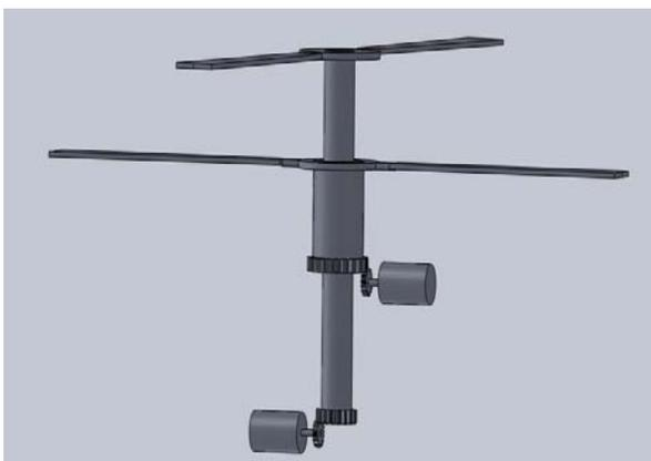
The following design shows the main rotor blades of the subsystem, where the upper blades are connected to the inner shaft and lower blades are connected to the outer shaft.
