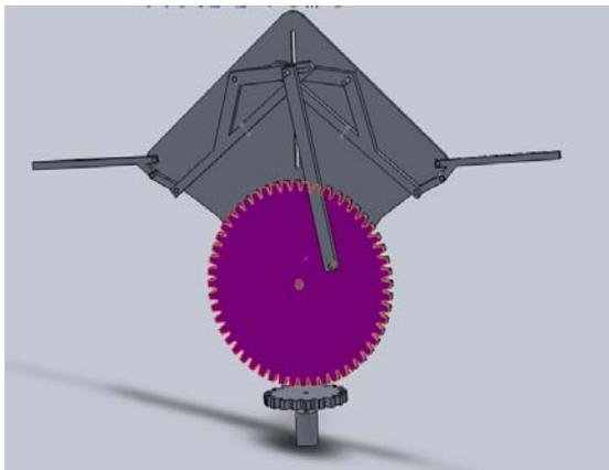
The following picture depicts the connecting system that has a connection with the main shaft that in turn is connected to the main gear.
