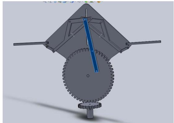
The following picture depicts the motor that is connected to the pinion gear which drives the main flap subsystem.
