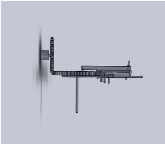
The following diagram describes about the main gear which is connected to the moving shaft of the system. The main gear is connected to the pinion gear located at the lower portion of the system.
