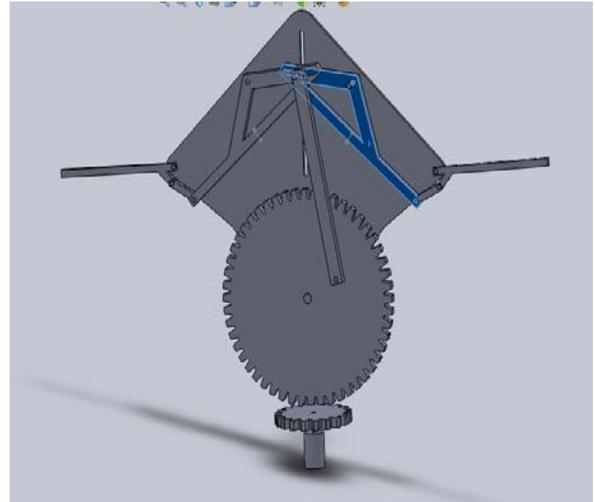
The following design shows the main connecting shaft, which connects the flaps and the main gear.
