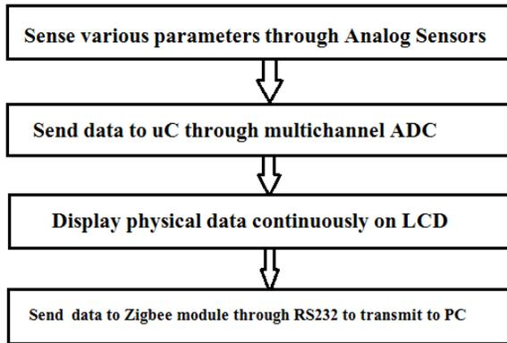
Figure. 3. transmitting flowchart
