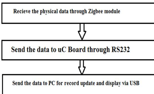
Figure.4. Receiver flowchart
