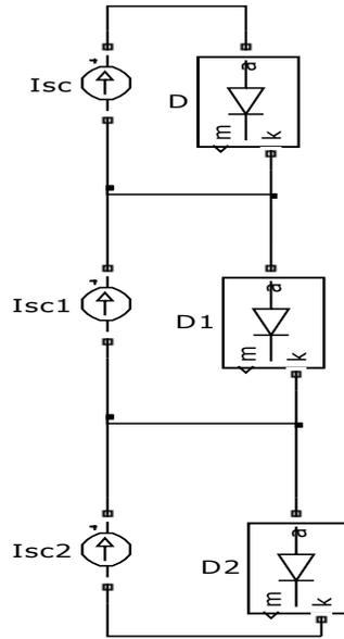
Figure 4.4 PV cell in series
