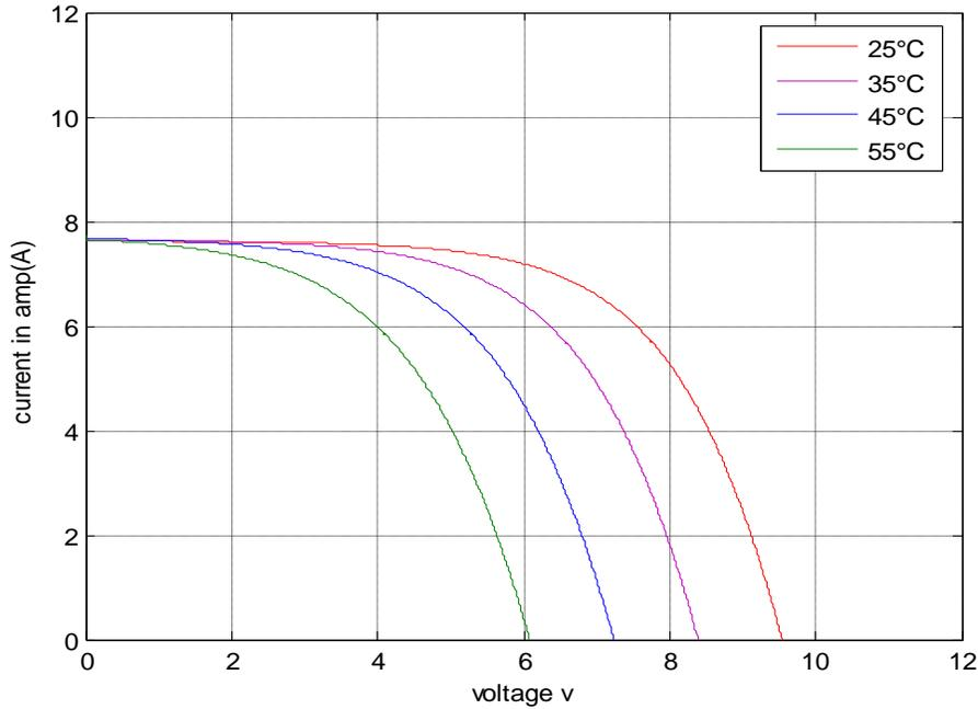
Fig. 5.1 (b) I-V characteristic of single diode PV cell with different temperature  $T_a$  ( $^{\circ}C$ )
