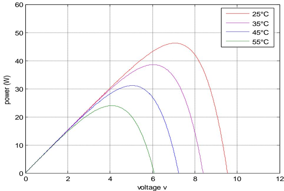
Fig 5.1 (d) P-V characteristic curves for the single diode PV cell with different temperatures  $T_a$  (°C)
