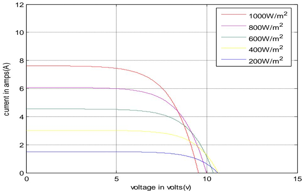
Fig.5.1(a) I-V characteristic of single diode PV cell with different irradiation  $G$  ( $\text{W/m}^2$ )
