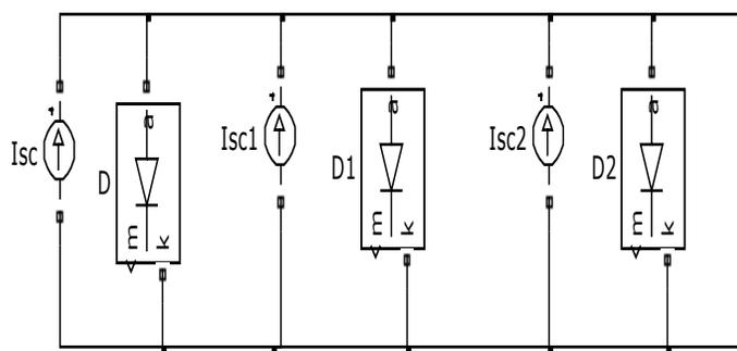
Figure 4.3 PV cell in parallel
