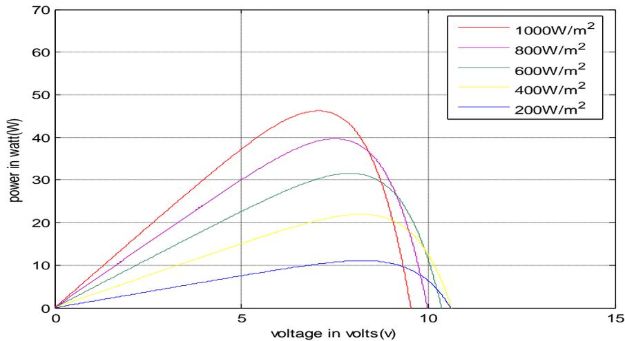
Figure 5.1 (c) P-V characteristic curves for the single diode PV cell with different irradiation  $G$  ( $W/m^2$ )
