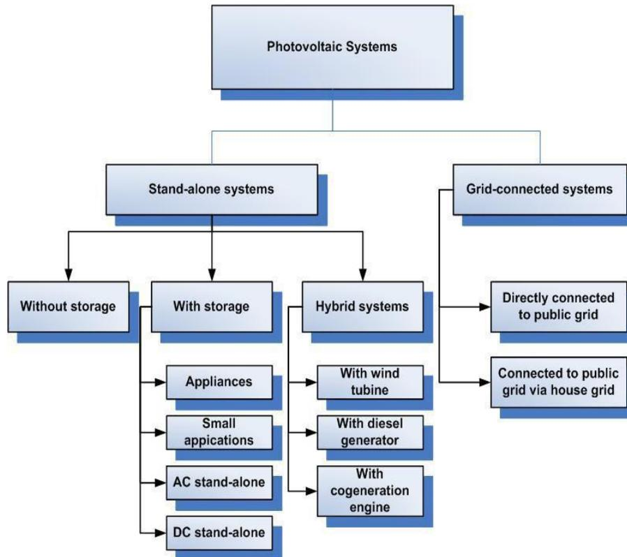
Fig 1.1 Classification of PV system
