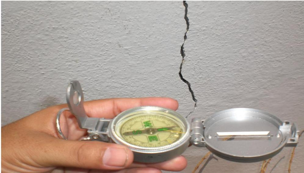
**Fig.1. Measurement of crack angle using compass**
