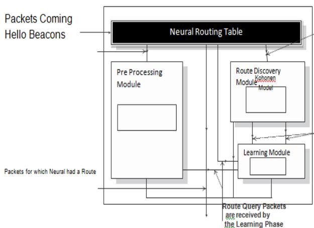
Figure 1. Schematic modular Architecture for NEURAL
