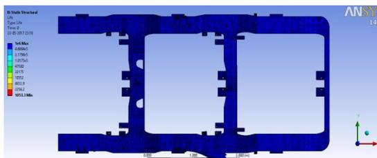
Fig. 4(a) Fatigue life analysis of Casting Bogie Frame
