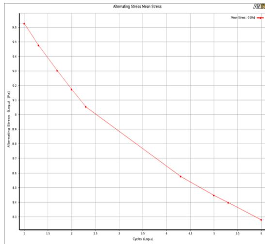
Fig 1(a): S – N Curve for Cast Steel
