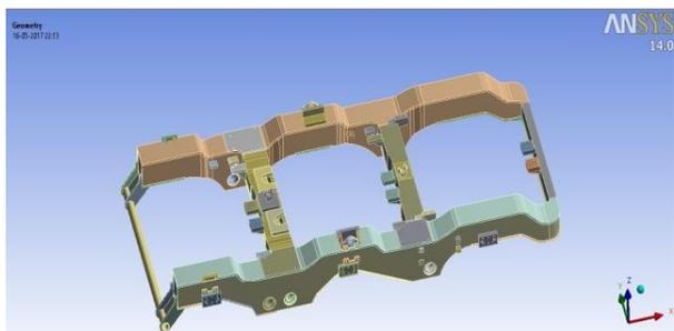
Fig. 2(b) Geometric Modelling of Bogie Frame (Fabrication Model)
