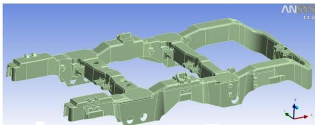
Fig. 2(a) Geometric Modelling of Bogie Frame (Casting Model)
