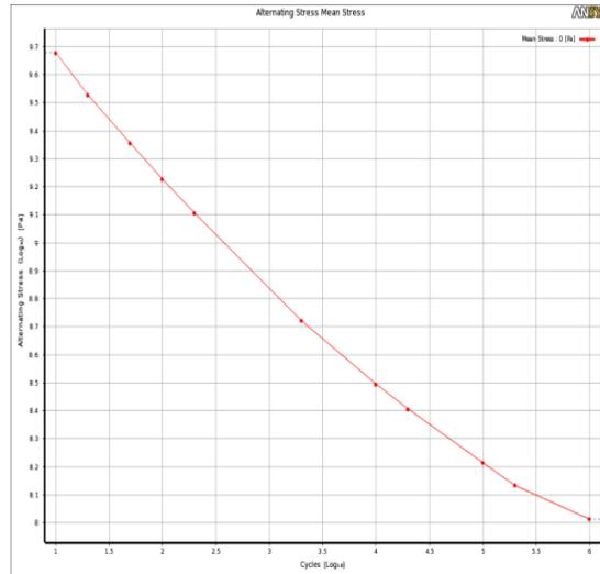
Fig 1(b): S – N Curve for E 350 C
