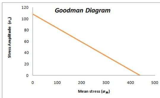
Fig. 3(a) Goodman Diagram of Cast steel
