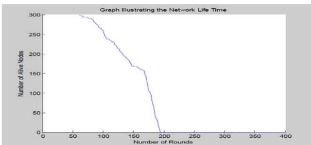
Fig 3. Network lifetime graph for First-level hierarchical Routing protocol
