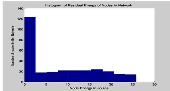
Fig 4. Histogram of residual energy for Non-hierarchical routing protocol
