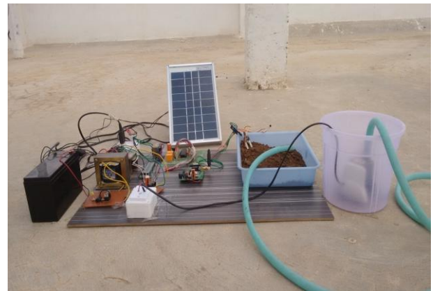
Figure8. Setup of Solar powered automatic irrigation system
