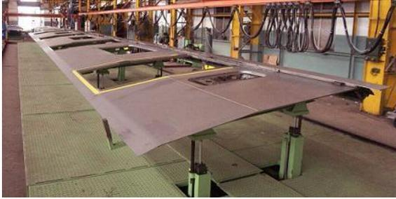
Figure 3.1: Sidewall assembly jig
