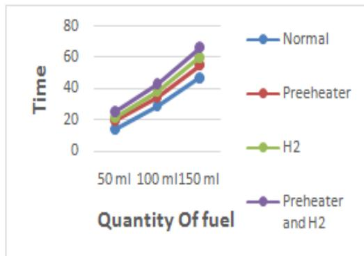
When test is carried out on experimental setup, obtained result is shown in graph. From above graph for the same quantity of fuel, running time of engine increases upto 10 minutes by implementing the preheater and electrolysis kit.
