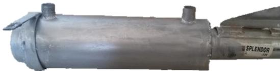
Fig 3.2 Heat exchanger mounted on silencer
