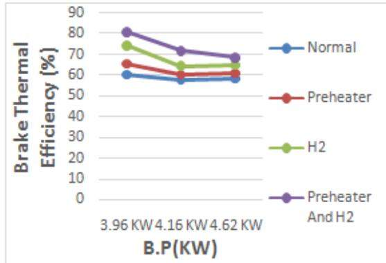
In normal condition brake thermal efficiency of the engine is low as shown in graph. When the preheater and electrolysis kit connected to the setup, mass of fuel is reduced. It is directly affected to the efficiency i.e. increase in brake thermal efficiency.
