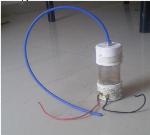
Fig 4.2 Hydrogen Generator
