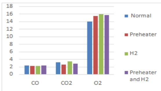
The above graph shows slightly reduction in CO (% volume) by connecting the preheater and electrolysis kit. It also shows reduction in CO<sub>2</sub> and slightly increase in
