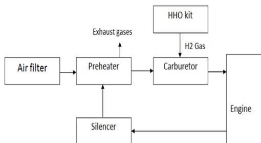
Fig 5.1 Block Diagram of Experimental Setup
