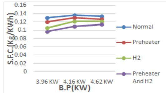
As shown in the graph specific fuel consumption is increases with increase in brake power. For normal condition, specific fuel consumption is higher than the other conditions. Use of preheater and electrolysis kit will reduce the specific fuel consumption as shown in graph.
