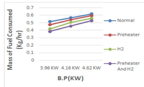
As shown in the grap hit is seen that Fuel consumption is increases as increase in Brake Power. But when the pre heater and electrolysis kit is connected to the engine, mass of fuel consumption decreases.
