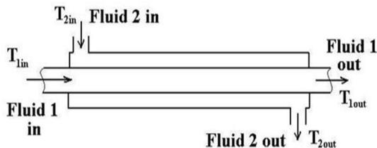
Fig 3.1 Parallel Flow Double Pipe Heat Exchanger
