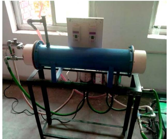
Figure 3: Shell and tube heat exchanger setup
