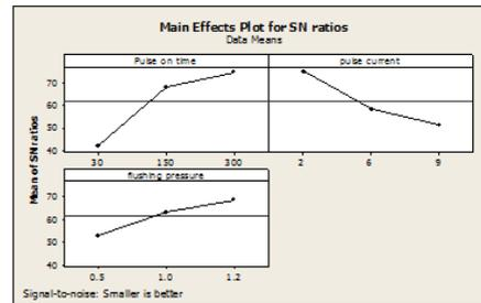
**Fig.5** Ratio curves of Process parameters of TWR for without heat treated tool
