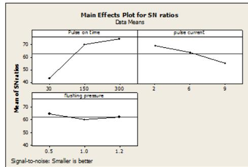
**Fig.8** Ratio curves of Process parameters of TWR for Heat treated tool
