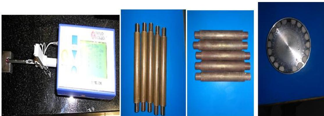
Fig.3(a) Profilometer (b) without heat treated and heat treated copper tool after machining (c) Workpiece(EN 8) after machining
