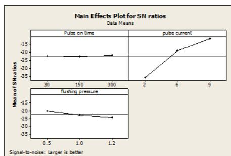
**Fig.7** Ratio curves of Process parameters of MRR for Heat treated tool
