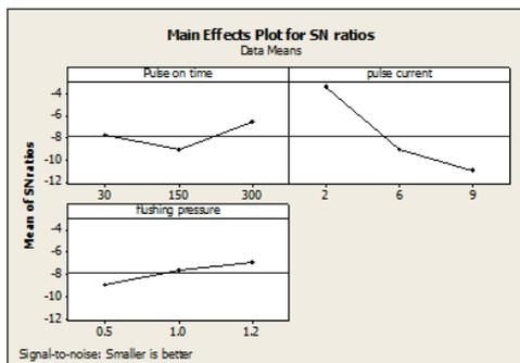
**Fig.6** Ratio curves of Process parameters of SR for without heat treated tool
