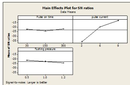
**Fig.4** Ratio curves of Process parameters of MRR for without heat treated tool
