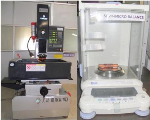
Fig.2(a) Die sinking EDM (b) Semi-micro balance
