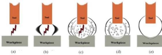
**Fig.1**(a) Pre-breakdown phase (b) Breakdown phase (c) Discharge phase (d) End of the discharge and (e) Post-discharge phase
