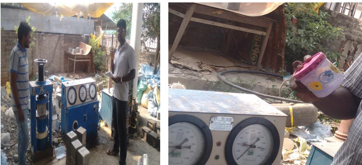
Fig 3: Testing of Cubes (boxes are 100% reusable)
