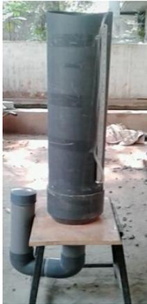
3.1 Falling head apparatus
