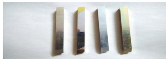
Fig. No 2 Single Point HSS cutting Tool (Left to right: Uncoated, Zn coated, Ni coated and Chromium Coated tool)
