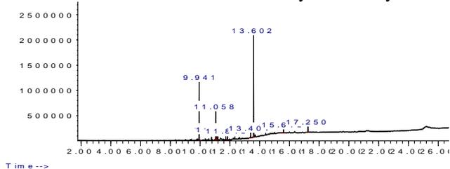
Figure 4: GC-MS results of methyl esters extracted using HCl as an osmotic agent
