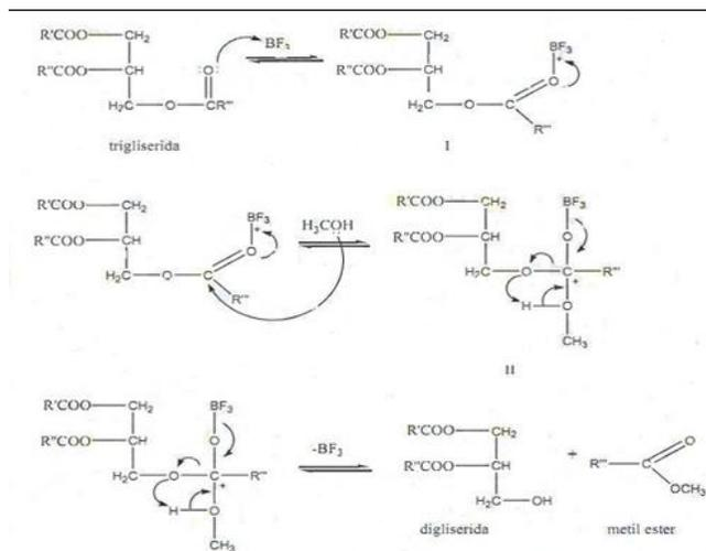
Figure 3: Esterification of triglycerides with  $\text{BF}_3$  methanol
