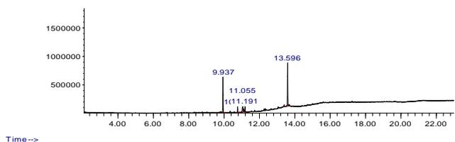
Figure 5: GC-MS results of methyl esters extracted using  $\text{CH}_3\text{COONa}$  as an osmotic agent
