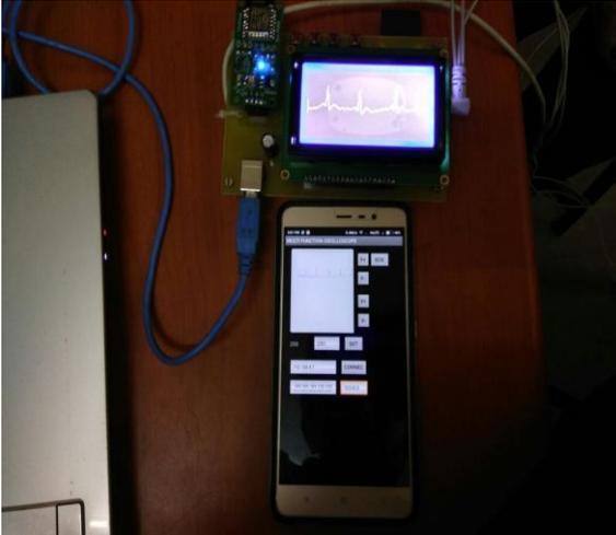
**Figure 6: ECG Recording and Display**
