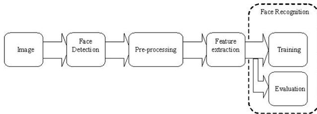
Fig. 4. Algorithm process
