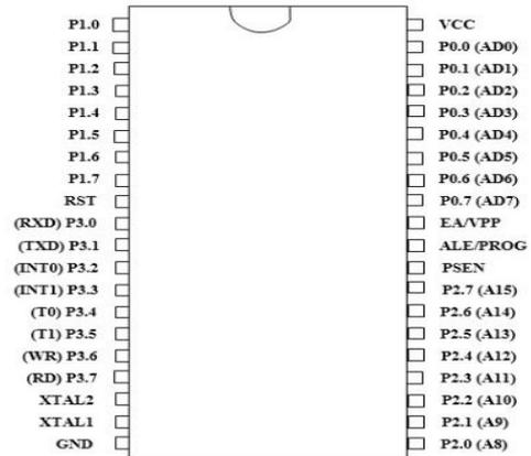
Figure3: Pin Diagram of 8051 microcontroller
