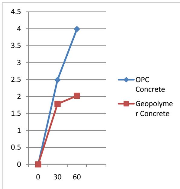
Graph 5.2: Comparison of weight loss of OPC concrete and Geopolymer concrete on sulphate acid
