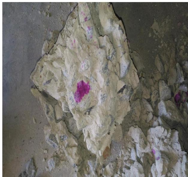
Fig 5.1- Carbonation test on concrete
