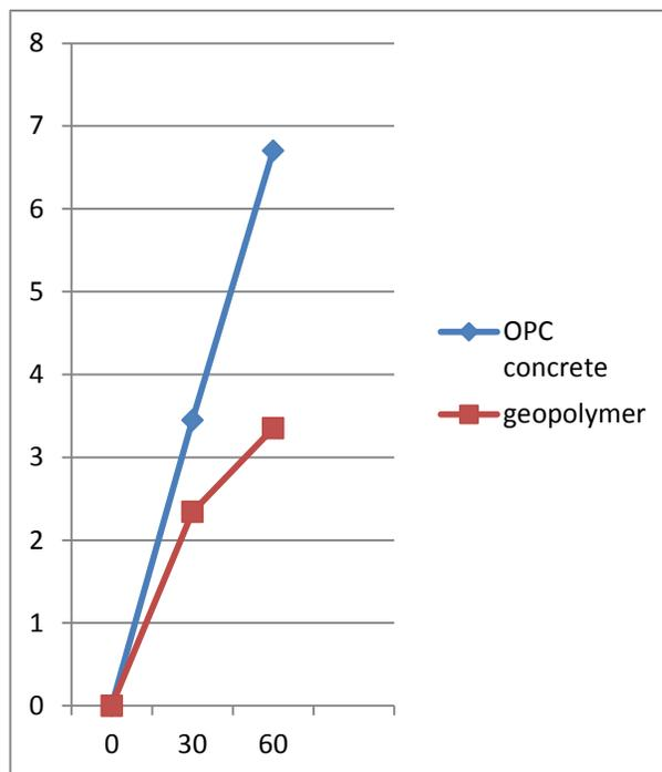
Graph 5.1: Comparison of weight loss of OPC concrete and geopolymer concrete on acid.
