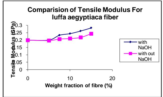
Fig7: Shows the Tensile modulus of luffa Fiber
