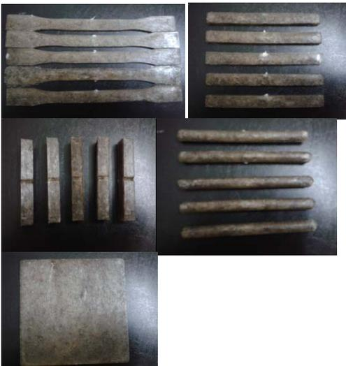
Fig3: Shows the Fabricated Composite Specimens to perform mechanical and machining characteristic
