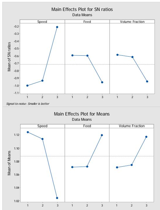
Fig15:shows the optimum cutting parameters for composite treated with NaOH
