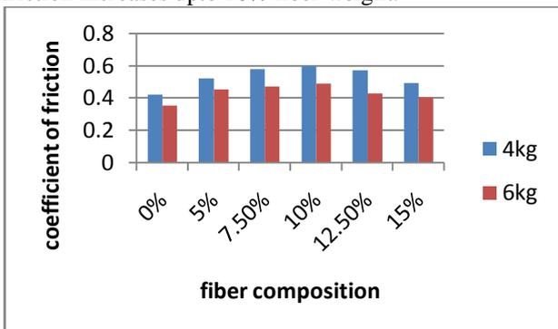
Fig12: coefficient of friction at different loads and composition at 100cm/s velocity
