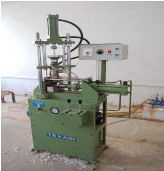
Fig2: Injection Moulding Machine
