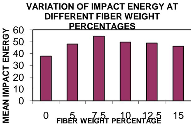
Fig11: Shows the Impact Strength of luffa Fiber treated with NaOH
