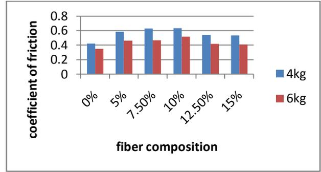
Fig13: coefficient of friction at different loads and composition at 100cm/s velocity treated with NaOH
