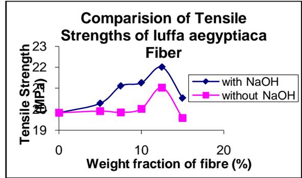
Fig6: Shows the Tensile Strength of luffa Fiber
