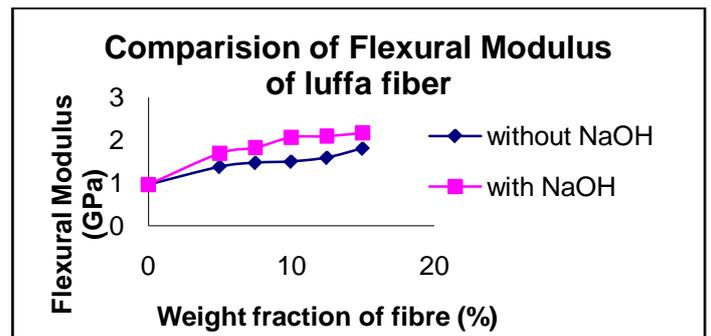
Fig9: Shows the Flexural modulus of luffa Fiber
