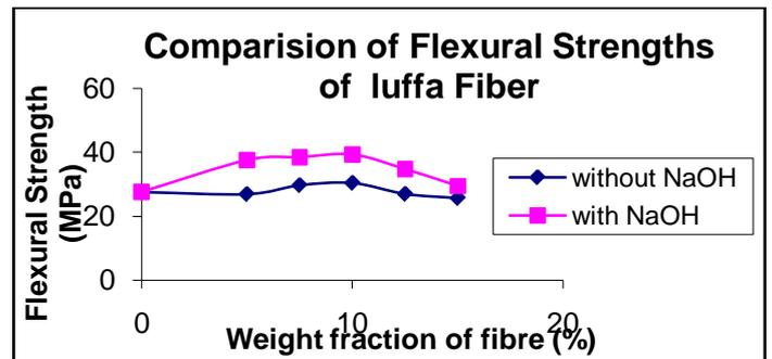
Fig8: Shows the flexural Strength of luffa Fiber
