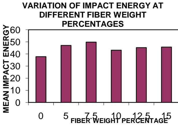
Fig10: Shows the Impact Strength of luffa Fiber
