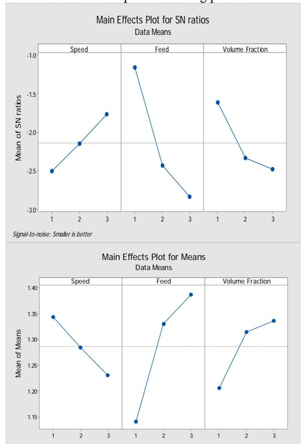
Fig14: shows the optimum cutting parameters
