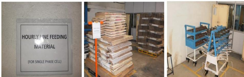
**Fig.2: Store prepares the trolleys with the materials according to the fixed quantity as per the released PRD. These trolleys are parked at a predefined location inside the stores.**
