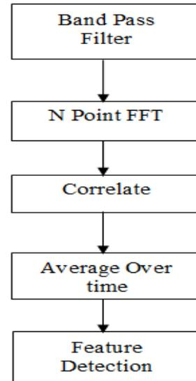
Figure.3: Block Diagram of CFD
