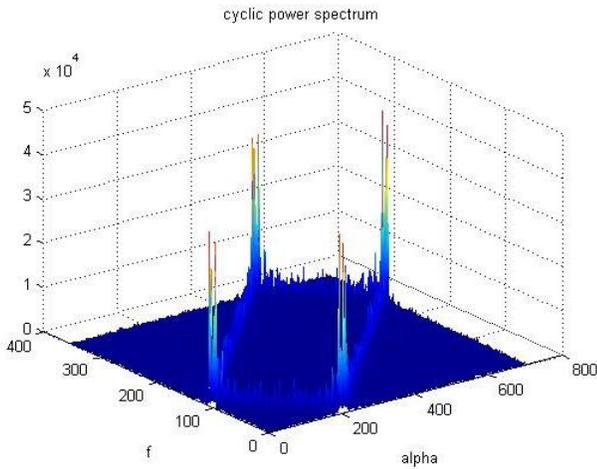
**Figure.5: Cyclic power spectrum for  $f=100$ MHz**
