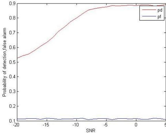
**Figure.6: ROC curve for SNR vs probability of detection, false alarm.**
