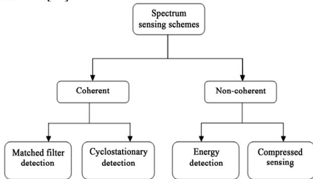
Figure.1: Types of Spectrum Sensing
