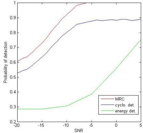
**Figure.7: ROC curve for SNR vs Probability of detection**
