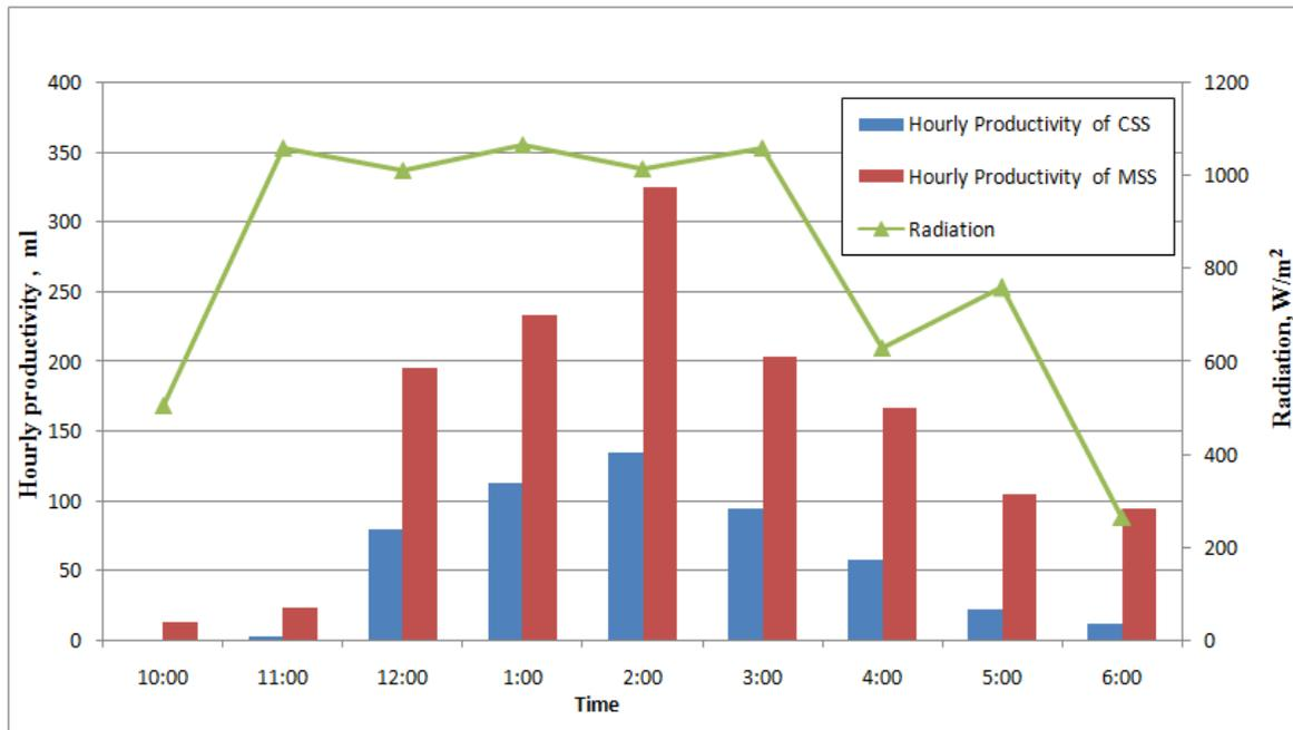
Fig.4. Comparison of hourly productivity of MSS and CSS with time
