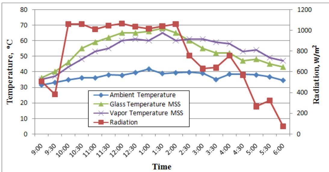
Fig. 3. Variation of MSS temperatures with time
