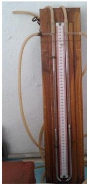
**Fig.5. U-tube differential manometer**
