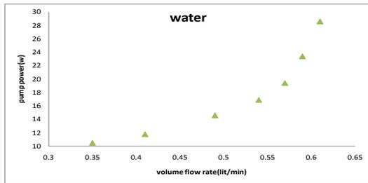
**Fig.8. Effect of volume flow rate of water on pump power**
