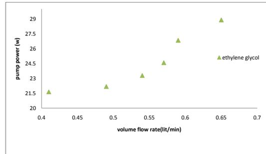
**Fig.10. Effect of volume flow rate of diluted EG on pump power**
