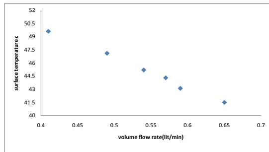
**Fig.9. Effect of volume flow rate of diluted EG on surface temperature**
