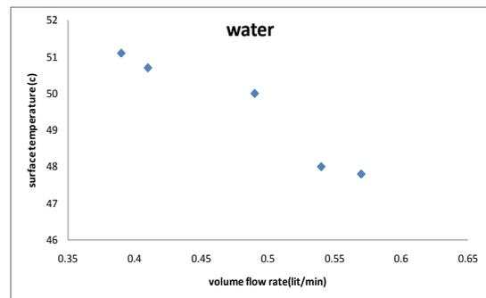
**Fig.6. Effect of volume flow rate of water on surface temperature.**
