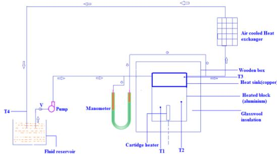
**Fig.1. Line diagram of Experimental setup**
