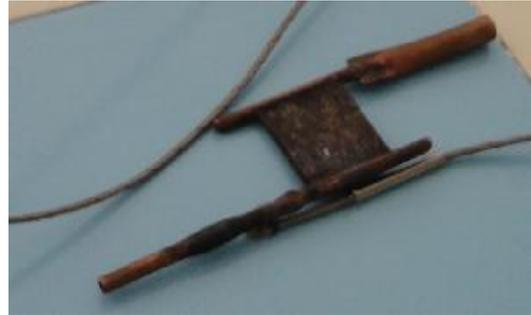
**Fig.2. Copper heat sink**
