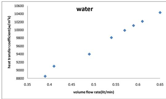
**Fig.7. Effect of volume flow rate of water on convective heat transfer co-efficient**
