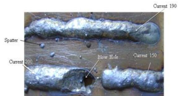
Figure 3: Pilot work on AISI 304
