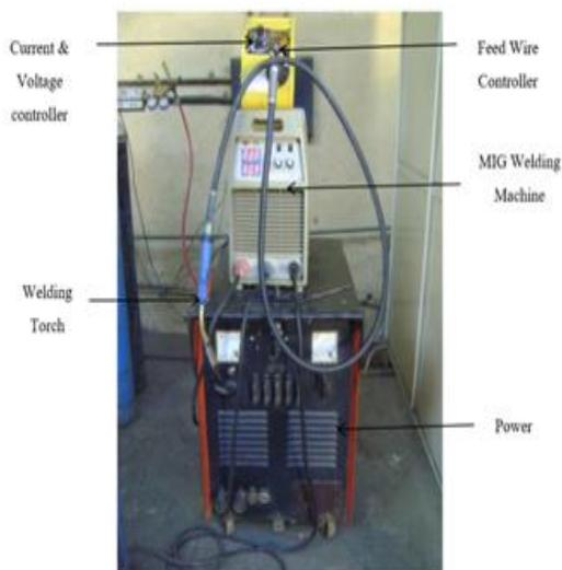
Figure 1: Gas metal arc welding setup
