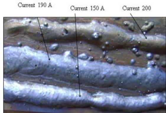
Figure 6: Weld bead using different shielding gas
