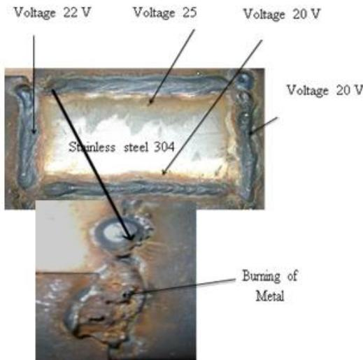
Figure 5: Blow hole in welding due to high voltage and current selected
