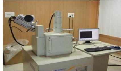
**Fig: Scanning Electron Microscope**
