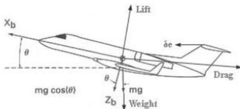
Fig.1. Description of pitch control system
