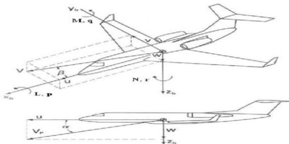
Fig.2. Definition of force, moments and velocity in body fixed coordinate
