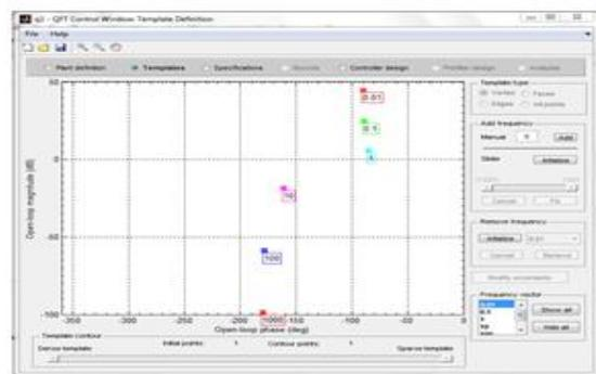
Fig.8. Plant template generation
