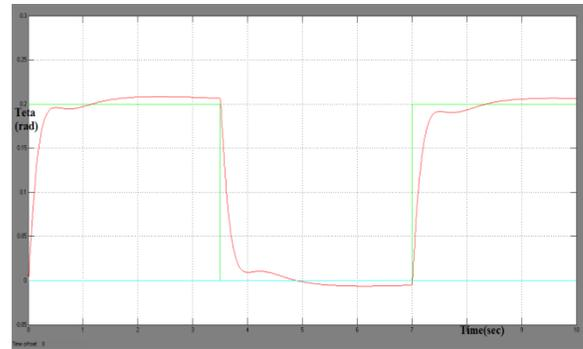
Fig.11. Pitch angle response with GA based QFT controller
