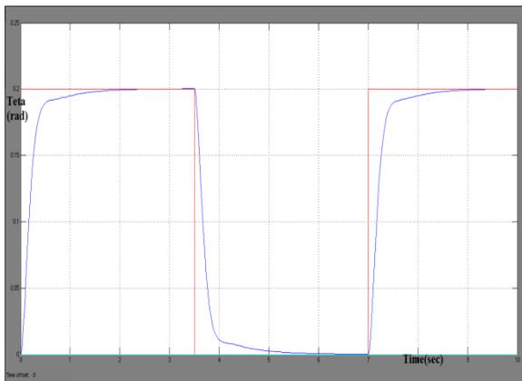
Fig.9. Pitch angle response with Self-tuning Fuzzy PID controller
