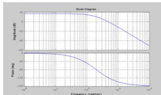
Fig. 7. Bode plot representation of P(s)
