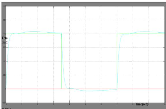
Fig.10. Pitch angle response with QFT controller
