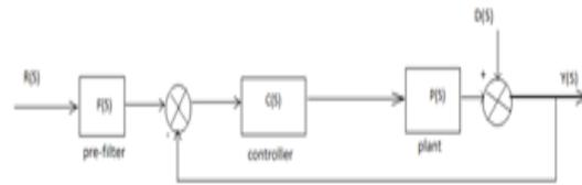
Fig.5. QFT Controller Design
