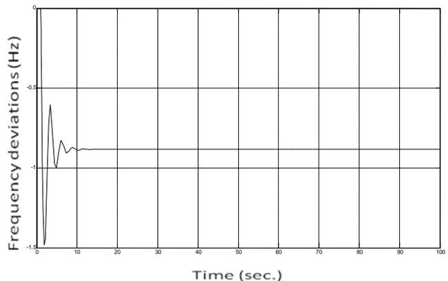
Fig 4 Result of Single area LFC without PI control
