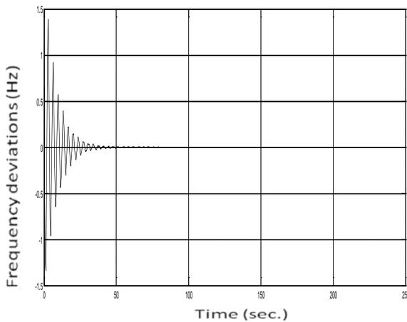
Fig 6 Result of Single area LFC with PI control
