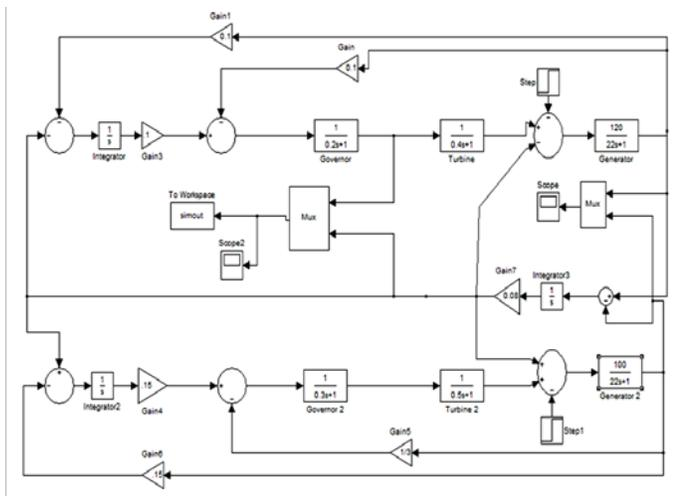
Fig 7 Simulation of double area interconnected power system
