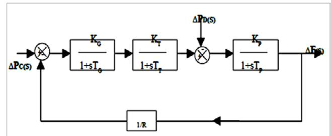
Fig:1 Block Diagram of a single area Power System for load frequency control
