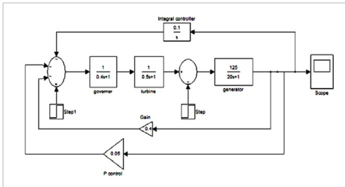
Fig 5 Simulation of Single area LFC with PI control
