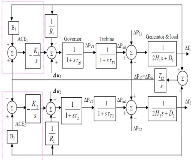
Fig:2 Block Diagram of a double area Power System for load frequency control
