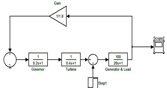
Fig 3 Simulation of Single area LFC without PI control
