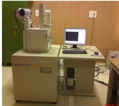
Figure 3: JEOL JSM-6480LV scanning electron microscope
