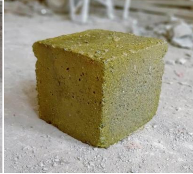
Fig 5.14 Acid affected cube
