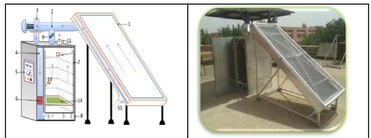
Figure 2: Schematic representation of the convective solar dryer.
