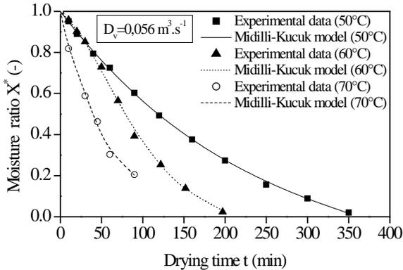
Figure 8: Experimental and predicted moisture ratios obtained using Midilli-Kucuk model
