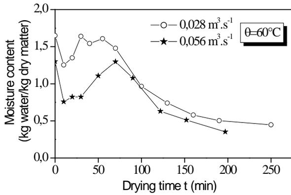
Figure 6: Variation of moisture content vs time for different drying air conditions
