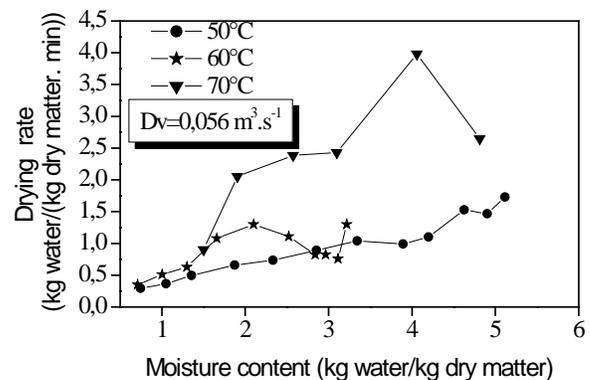
Figure 5: Drying curves of *Z. gaetulum* at different temperatures
