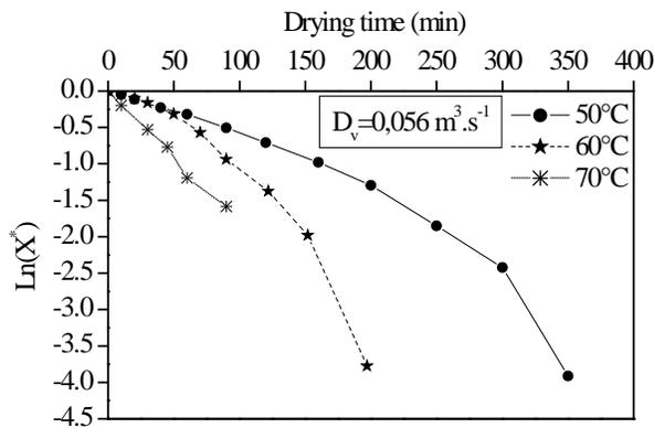
Figure 9b: Plot of  $\ln(X^*)$  vs time for different drying air conditions
