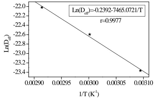
Fig. 10: Influence of drying air temperature on the effective diffusivity.
