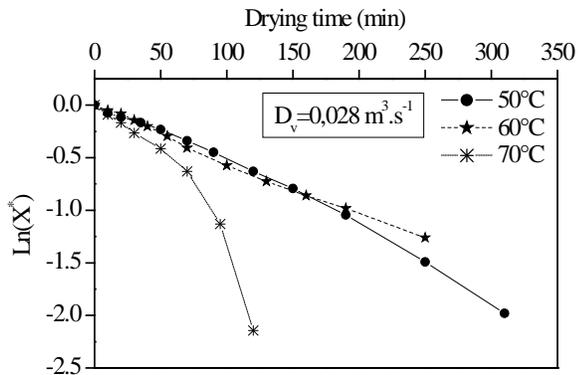
Figure 9a: Plot of  $\ln(X^*)$  vs time for different drying air conditions
