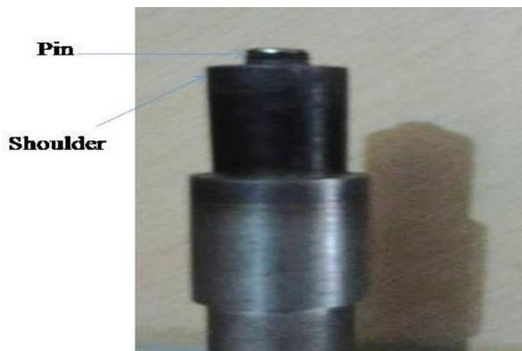
**Figure 2: Welding tool profile**
