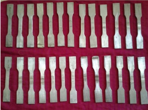
Figure 5: Specimens before testing
