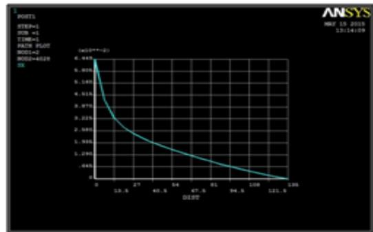
Figure 6: Variation of radial stress for linearly varying disk
