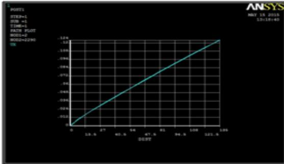
Figure 2: Variation of radial displacement for uniform disk
