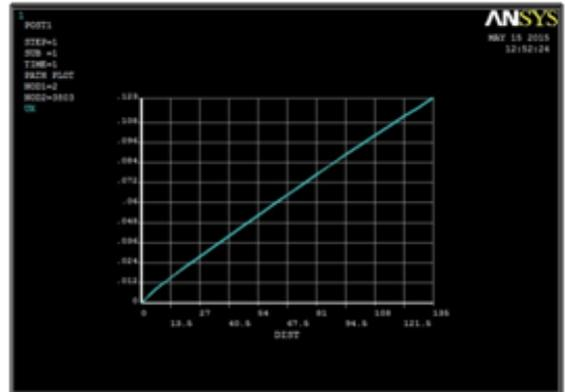
Figure 11: Variation of radial displacement for concave disk
