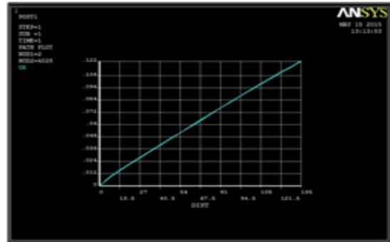
Figure 5: Variation of radial displacement for linearly varying disk
